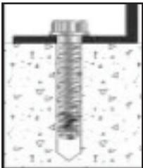
8. Be sure the anchor is at the required embedment depth and the maximum torque has not been exceeded (50 ft. - lbs.).
