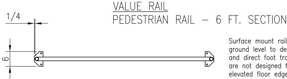
Surface mount railing used at ground level to define areas and direct foot traffic. Rails are not designed for use on elevated floor edge.
